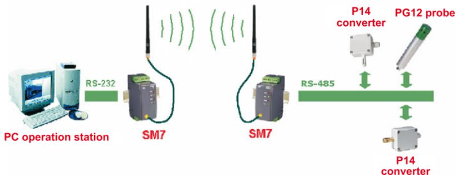
**Fig.1. Exemplary monitoring of temperature, humidity and pressure**
